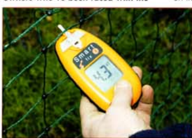
A voltmeter is essential for monitoring system efficiency. This one costs about £60.
