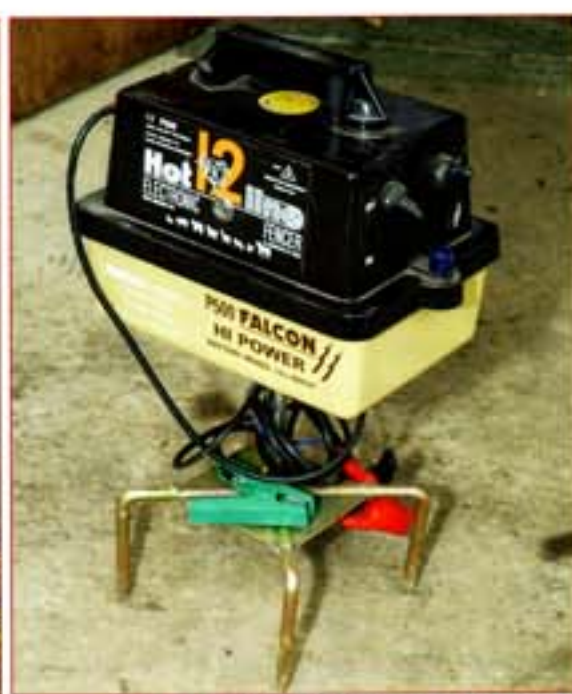
Stand-alone systems use 12-volt leisure/caravan batteries rather than automotive units. They offer great portability and operational flexibility, but need to be regularly charged.
